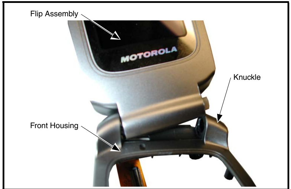
Figure 12. Removing the Flip Assembly
